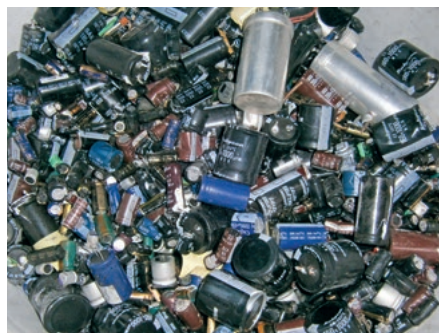
Condensers from manual dismantling
