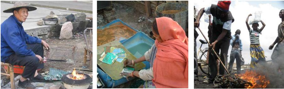
**Fig. 2.** Typical recycling processes applied in the informal sector of developing countries (left to right: de-soldering of printed wiring boards, leaching of gold from printed wiring boards, open burning of cables) (Pictures: Empa)
